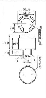
These electromagnetic transducers are really subminiature loudspeakers. Being lower impedance than piezo devices, they offer better sound output at low drive voltages - down to 1.1V peak to peak. Output will be highest at the resonant frequency, but reasonable response over the audio range allows multi tone or low fidelity speech reproduction. The QMT111 is a very popular low cost transducer suitable for 5V square wave operation.
