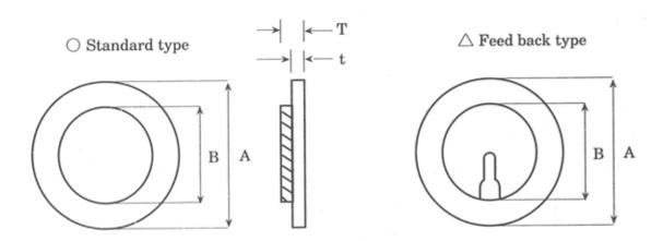
Piezo elements are the basic sound generator in all piezo devices. They are a very economical, super-thin sound transducer, and are also commonly used in reverse, as a shock / vibration sensor in security applications.
