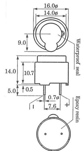
These electromagnetic transducers are really subminiature loudspeakers. Being lower impedance than piezo devices, they offer better sound output at low drive voltages - down to 1.1V peak to peak. Output will be highest at the resonant frequency, but reasonable response over the audio range allows multi tone or low fidelity speech reproduction. The QMT111 is a very popular low cost transducer suitable for 5V square wave operation.
