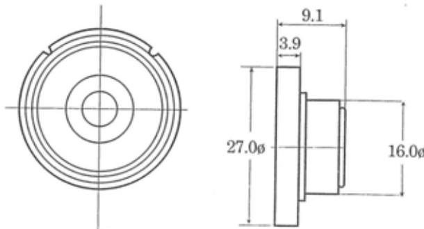
These are miniature polymer cone dynamic loudspeakers commonly used in phone or audio equipment monitor situations. They offer good sound fidelity over the stated frequency range and can be driven by low level low impedance signals.
