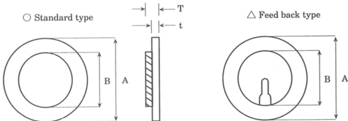
Piezo elements are the basic sound generator in all piezo devices. They are a very economical, super-thin sound transducer, and are also commonly used in reverse, as a shock / vibration sensor in security applications.
